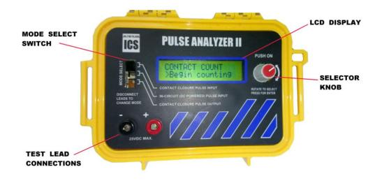
The above diagram illustrates the connection points and switches on the PA1 pulse analyzer.
